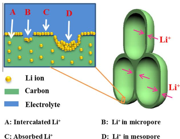
Fig. 8. Schematic of lithium storage and transport in PACS.
